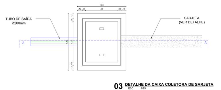
**03 DETALHE DA CAIXA COLETORA DE SARJETA**
